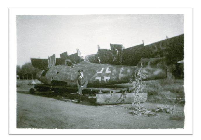
This abandoned Messerschmitt Me 262A, appears to have a large light colored "I" with a dark "7" near the tail, serial appears to be 418 543. It was being moved by road when the war ended, possibly being used by 9 Staffel, Jagdgeschwader 7, in the last Defence of the Reich. If that is the case the rear fuselage contained a front blue band, followed by a red band, and painted over the middle would be a large yellow "I". Seems to fit, however I am not a Luftwaffe markings expert.
